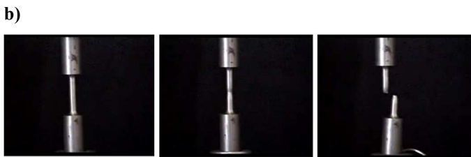
Fig. 2. (a) Accessing experiment raw data after completion of the tensile test. (b) Progression of the steel 1010 tensile test highlighting different physical stages of tensile test, such as necking (middle image).
